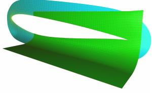
*Example of wall treatment on the fuselage/collar zone of a CRM configuration when output\_type is 2: if the collar is prioritized (middle) or not (right), the part of the fuselage falling inside the wing is clipped.*
