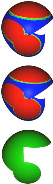
*From left to right: Sphere made of 2 overset patches, results with output\_type=0,1 and 2 displayed for the non-prioritized patch.*
